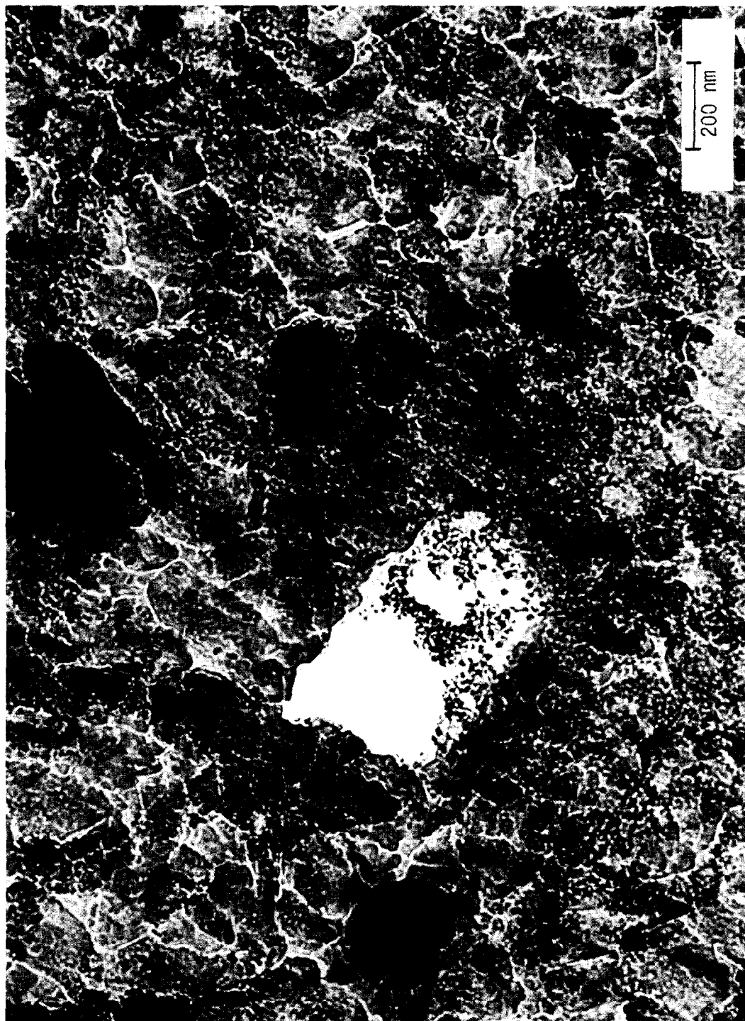
Fig. 2. Micrograph of the sintered catalyst regenerated for 1 h at 506°C.
